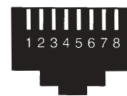
USOC RJ61 8 position/8 wire
