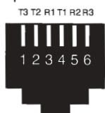
USOC RJ25 6 position/6 wire
