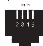
USOC RJ11 6 position/2 wire
