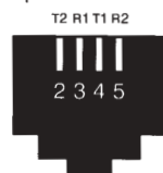
USOC RJ14 6 position/4 wire
